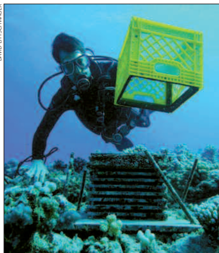
Chris Meyer recovering autonomous reef monitoring structures in Mo'orea, French Polynesia
