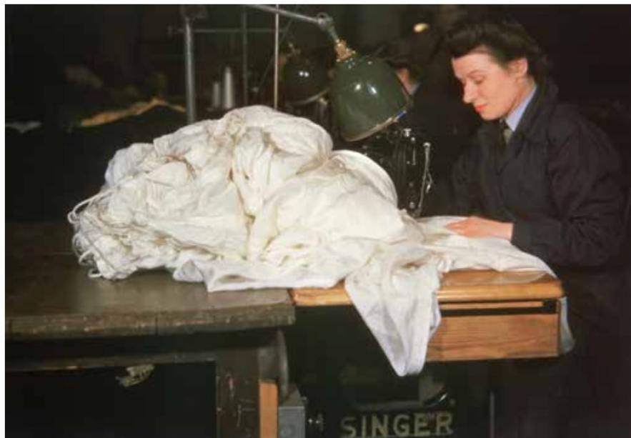
A member of the Women's Auxiliary Air Force uses a Singer sewing machine to stitch a bundle of parachute silk, circa 1942.
