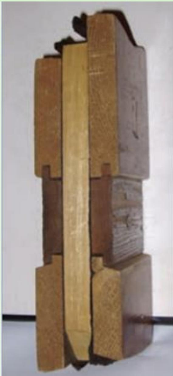
Sample of the 'Board-and-Batten' Sandwich-Wall
