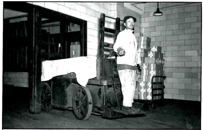
Battery-powered baggage trucks served as shopping carts to transport foodstuffs to diners. This one is exiting NYC's Mott Haven Commissary on July 28, 1943. NYCSHS Archive Image WR310664.
