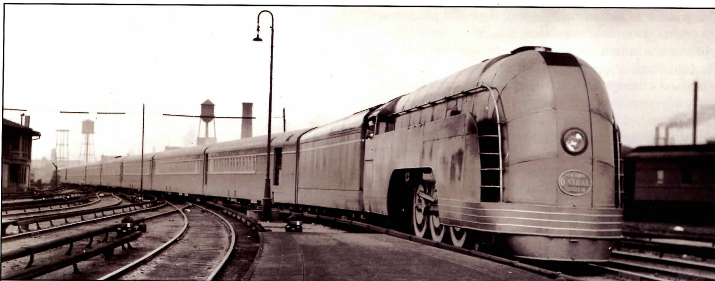
It's mid-morning in Detroit, and No. 750, The Mercury , rolls into a platform track with a nine-car train that originated, as No. 75, at Cleveland Union Terminal a little less than three hours earlier. The power is one of two K-5b Pacifics, largely concealed beneath a streamlining cowl born on the drawing board of famed industrial designer Henry Dreyfuss. Photo by G. Grabill, Jr., NYCSHS Archive Image PB405012.
