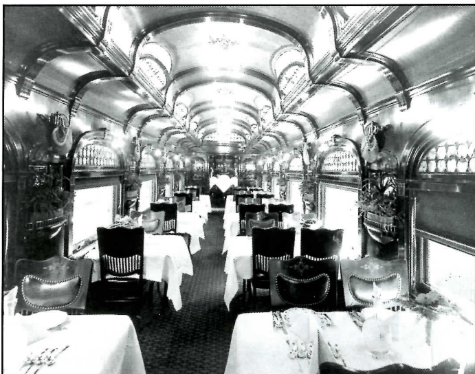
Some measure of the opulence of earlier New York Central dining cars may be gleaned from this interior view of a diner on the original 20th Century Limited of 1902. The offset aisle between tables for two and tables for four would be standard for many years. Jeff Hands Collection, NYCSHS Archive Image PB596094.
