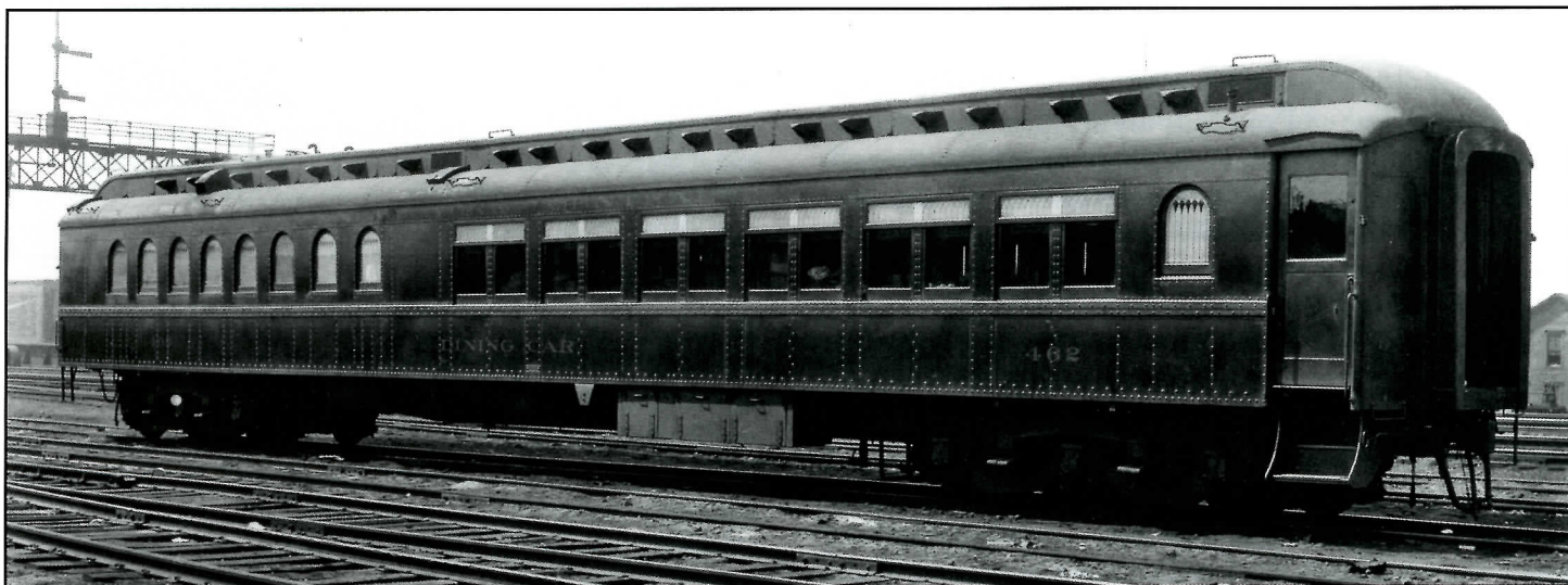
Arched and transom windows were still in vogue on steel diners when NYC 462 was built in 1920 as one of five cars in Lot 917 by Central's West Albany Shops. Originally seating 36, the car was later converted to a diner-lounge. It was renumbered to NYC 537 and, as X-23304 went into non-revenue service in October 1952, and was retired in February 1956. Car history courtesy of Hugh Guillaume. NYCHS Archive Image PB513027.
