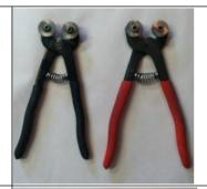
**Glass Scorer** For stained glass, carbide wheel scores glass, oil helps wheel score smoothly *Stained glass stores, on-line*
