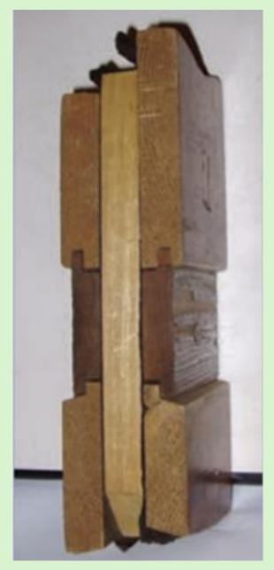
Sample of the 'Board-and-Batten' Sandwich-Wall
